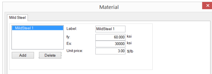
Figure 6.1-2 - Non-Prestressed Steel Dialog Box
